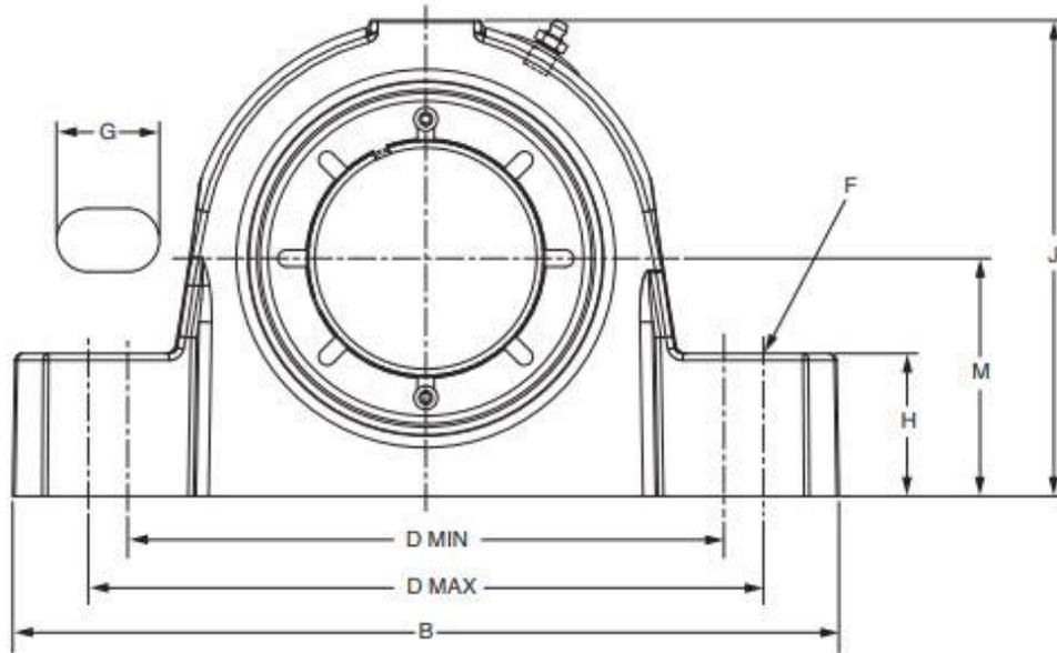
**NOTE:** All sizes use a 1/8-27 NPT hydraulic grease fitting
