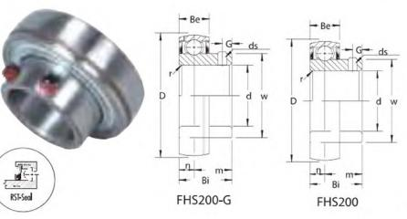
Standard load capacity Narrow inner ring with spherical outer ring Relubrication aroove with oil hole on set screw side(Shown) Oil hole opposite groove makes it interchangeable with all manufacturers (shown) Non-relubricatable bearing available (omit "G" from bearing part number) Nylon patched class 3A set screws are standard Standard seal: RST tight riding, full cover, metal shroud seals
