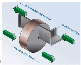
releases the adsorbed moisture into the heated regeneration air stream which is then exhausted to the outside.
