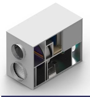
The 300 DES/DX desiccant-based dehumidifier is designed specifically for light commercial applications. The unit combines the benefits of both desiccant dehumidification and DX cooling to achieve the most energy efficient dehumidification. Waste heat is captured from the condensing coil and used to regenerate the desiccant rotor in order to provide further dehumidification.
