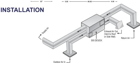
The 300 DES/DX is typically installed as shown with its own return air and supply ducts. The supply air ducts is branched to two or three supply air ducts servicing main rooms of the building. The 300 DES/DX is controlled by a separate humidistat and will cycle on and off to control humidity independently of the main A/C system.
